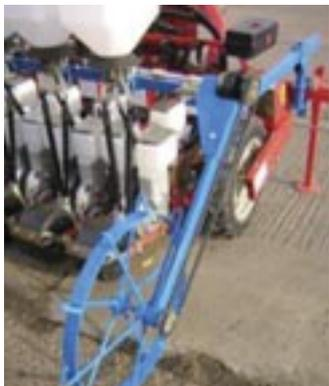
**Below right, close up of Horstine Farmery clutch fitted to sprocket drive.**
