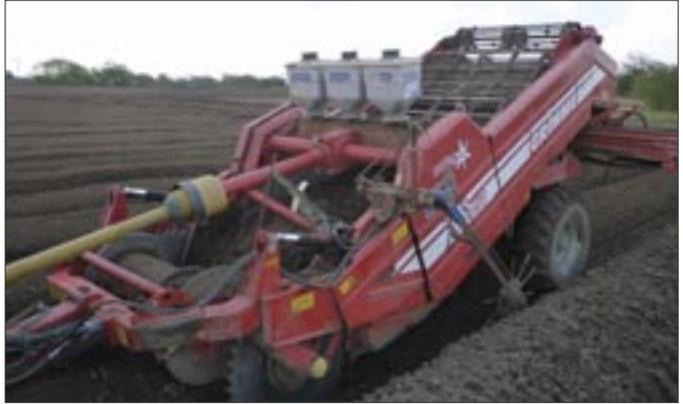
Not only do stars fail to mix the soil and nematicide granule but the design often prevents the applicator outlets being close to the share at the front of the machine.
