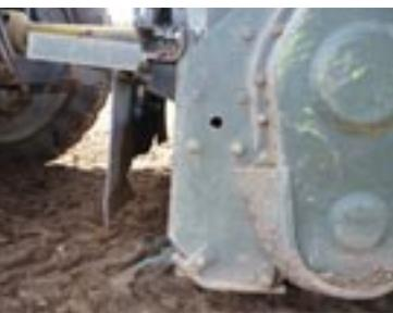
Exposed granules may pose a risk to wildlife. To prevent granules being left on the soil surface at row ends, shut-off the applicator two to three meters from the end of the working strip. This ensures that all granules have left the delivery tubes by the time the machine is lifted from the soil. A land-wheel continuing to turn after the applicator has been lifted out of work will cause product to be applied to the soil surface.
