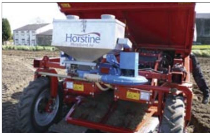
New product introductions such as those shown above are designed with operator use in mind. As you can see, the applicator unit can be filled at ground level rather than requiring the operator to climb on the machine.
