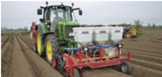
If applying Vydate® via a front mounted applicator and bed tiller ahead of the planter, ensure that the working depth of the bed tiller is at least the same depth as the planter 'shoe' opening the ridge on the planter. This will ensure untreated soil from below the treated zone is not lifted back into the final planted ridge.
